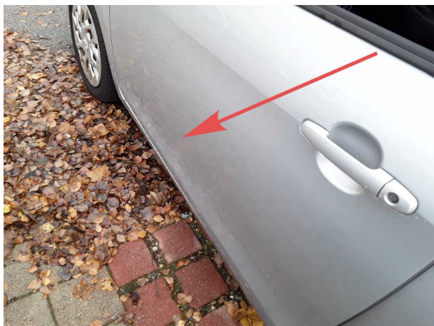
Beschädigung #8: Tür vorn links: Tür - Delle(n) - Smart Repair
