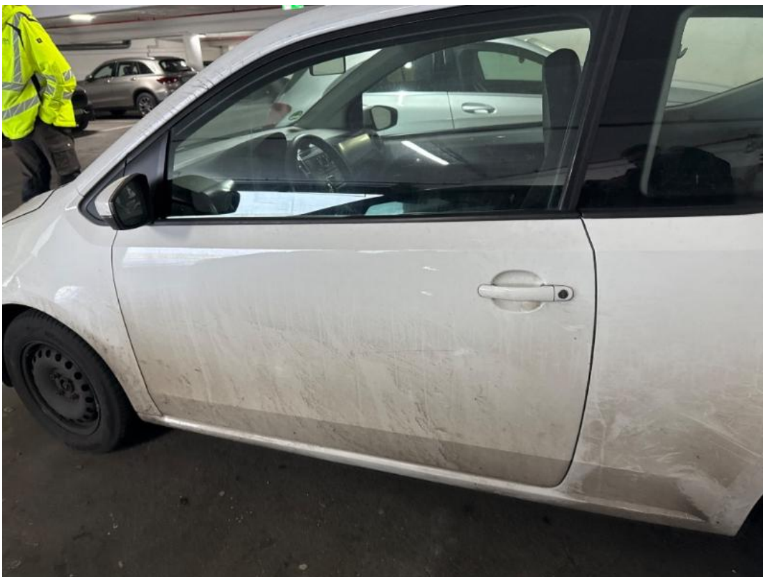
6. Tür vorne links - Kratzer
