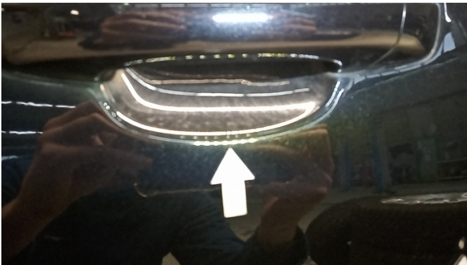
6. Tür Vorne - Links Kratzer -
