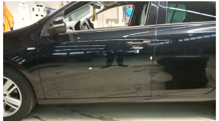
6. Tür Vorne - Links Kratzer -
