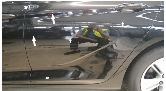
8. Tür Hinten - Links Kratzer -
