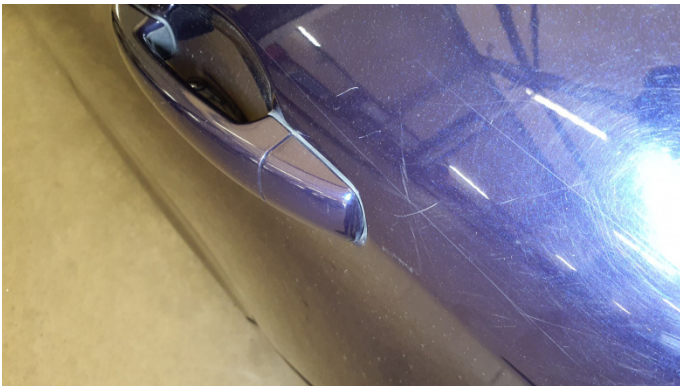
12. Tür Hinten - Links Kratzer -
