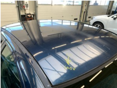
Roof - Hail damage
