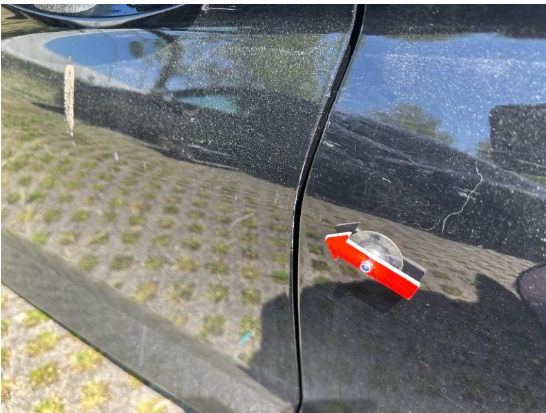
2. Tür vorne links - Kratzer
