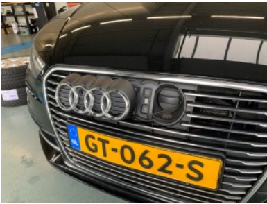
Laadpoort Vergrendeling Defect
